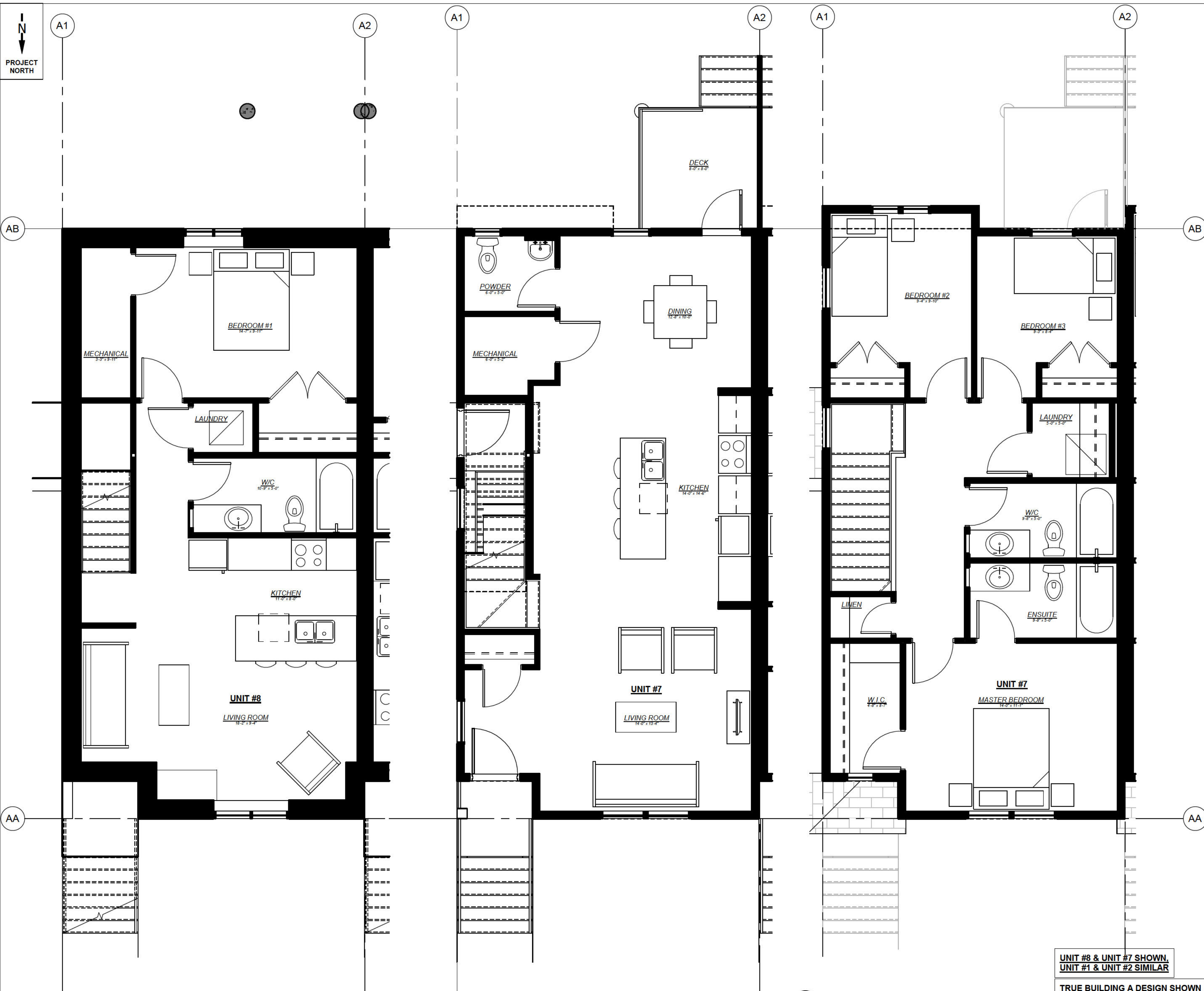
3 ENLARGED PLAN - UNIT #7 - SECOND FLOOR (ENDS) Scale: 1/4" = 1'-0"
